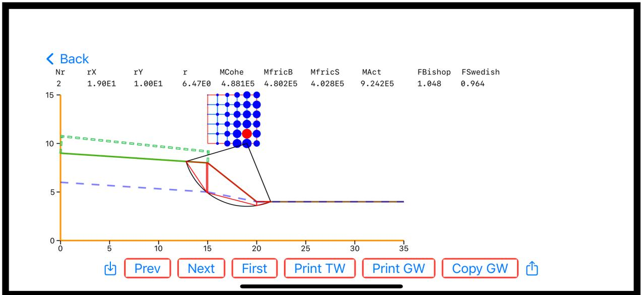
Figure 6: Another failure arc than the one with lowest safety factor analysed (from file Example 1)
