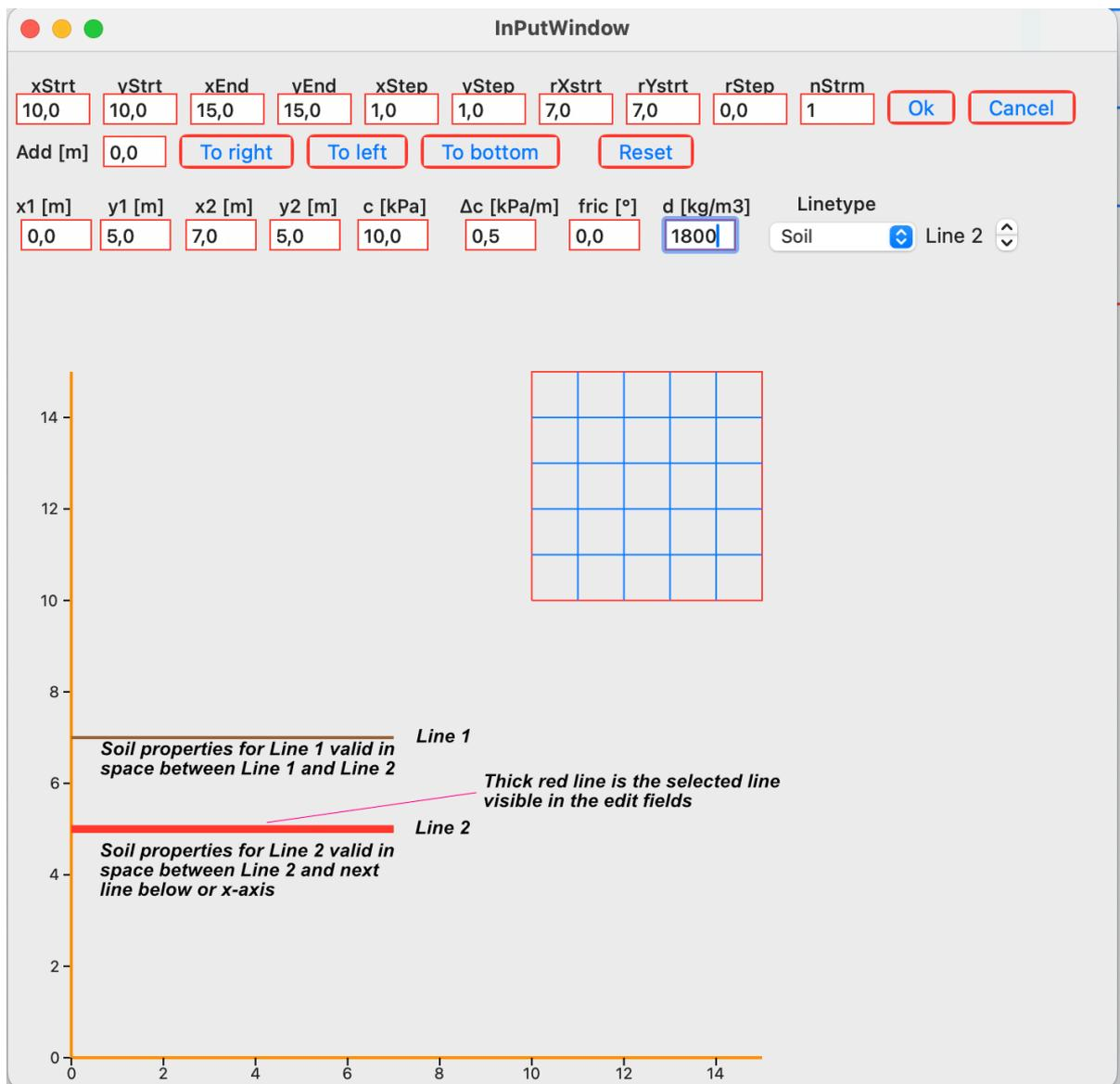
Figure 10: Example of Soil-lines and how they are defined. The Soil-properties present in the edit fields are valid until the next soil-line (Line 2).
