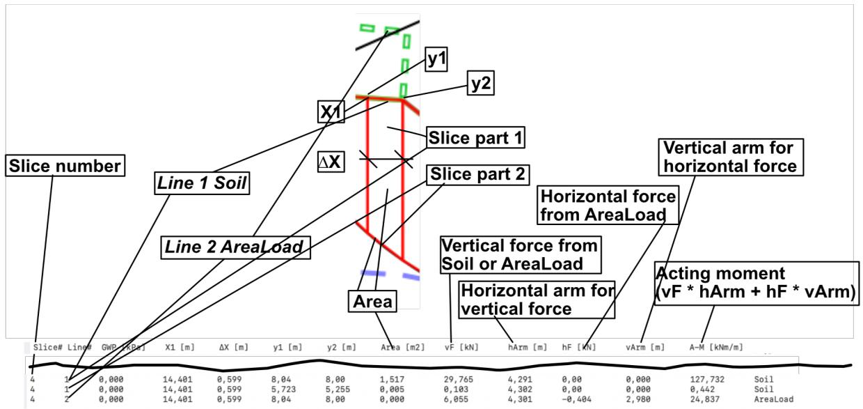
Figure 19: Explanation of output for slice 4 with line 1 governing the material properties. The slice contains slice part 1 and slice part 2 and AreaLoad from line 2. Text output from Example 1 but with  $nStrim = 10$ .
