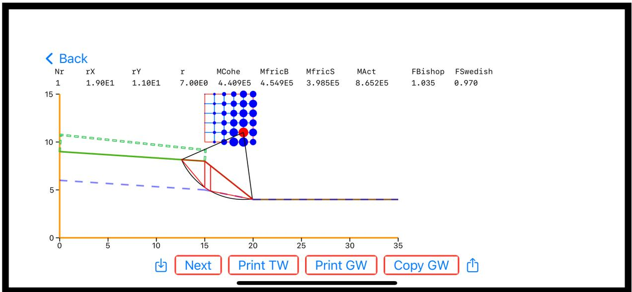
Figure 4: Screen after “Run slope” executed (from file Example 1).
