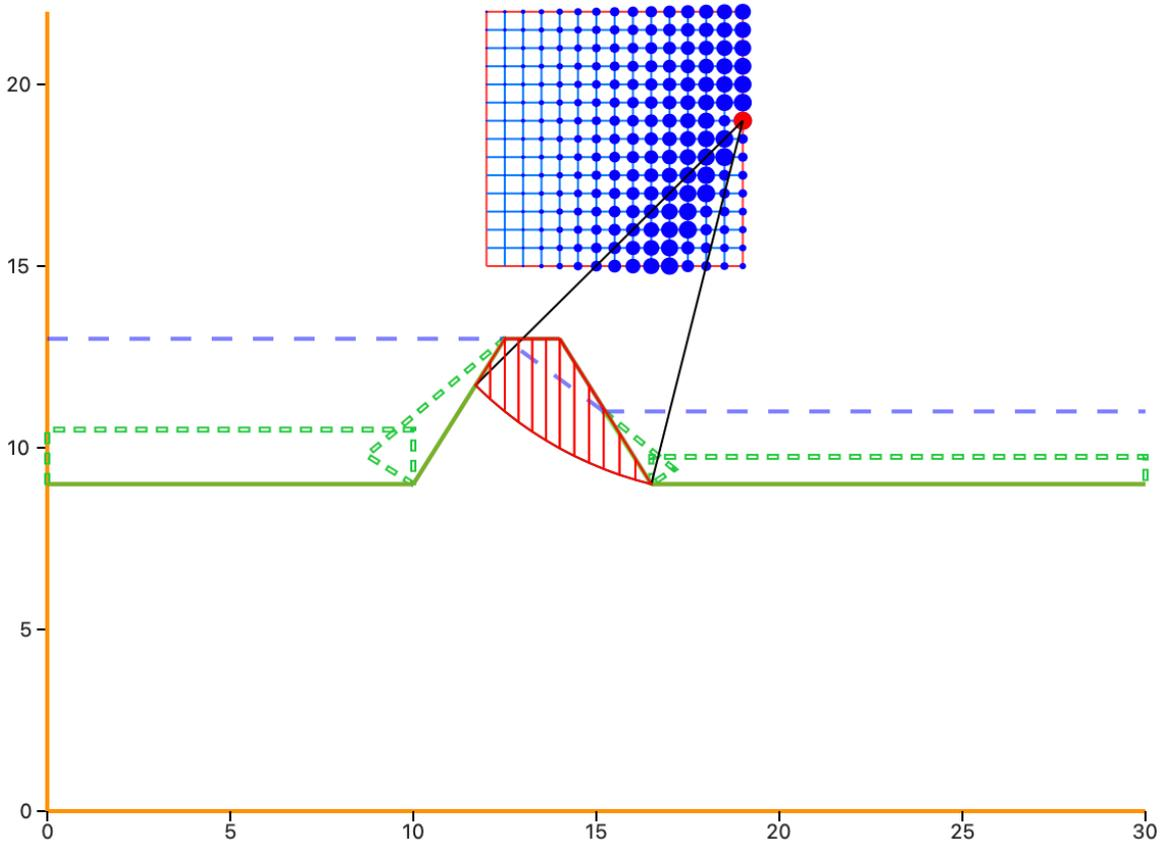
Figure 21: Display of critical center's. The red dot represents the most critical centre found. The bigger dot the more critical centre. The used search square seems to be a little bit too much to the left and probably a bit low.
