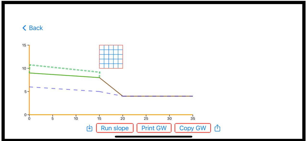
*Figure 3: Main action screen (GraphWindow) with action buttons before Run slope is executed (from file Example 1).*
