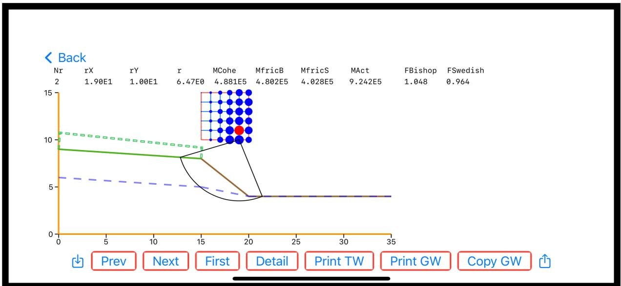
Figure 5: Examination of other failure arcs than the one with lowest safety factor according to simplified Bishop’s method of slices (from file Example 1).
