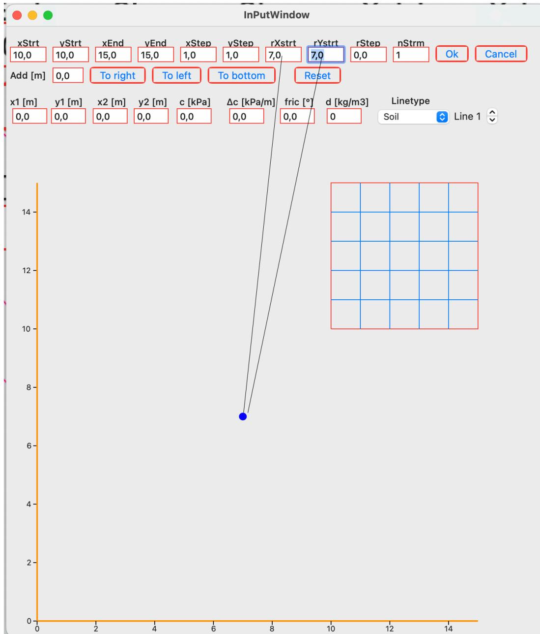
Figure 9: When a new set of calculations starts at a fresh centre the program must know where to place the first slope-circle. The point defined with  $rX_{strt}$  and  $rY_{strt}$  will be intersected with the first slope-circle.
